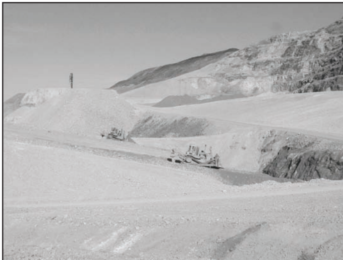
FIGURE 20.5 Equipment sloping backfill material in the Gold Bug pit, Zortman–Landusky mine, Montana
